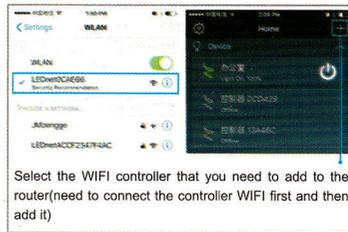
Select the WIFI controller that you need to add to the router(need to connect the controller WIFI first and then add it)
